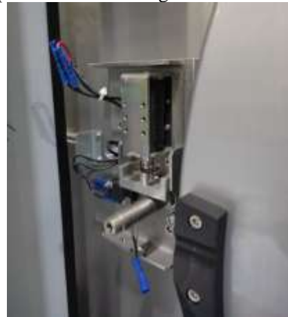
Figure 7. The tested solenoid-based door locking mechanism, showcasing its compact design and robust construction during mechanical durability testing.
