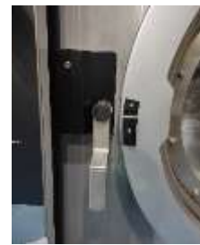
Figure 2. Close-up view of the washing machine door and the solenoid-based locking mechanism
