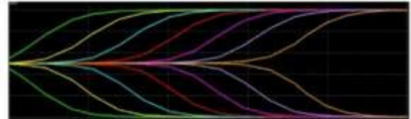
Figure 10: Output Signal Stabilization at Different Setup and Hold Times.
