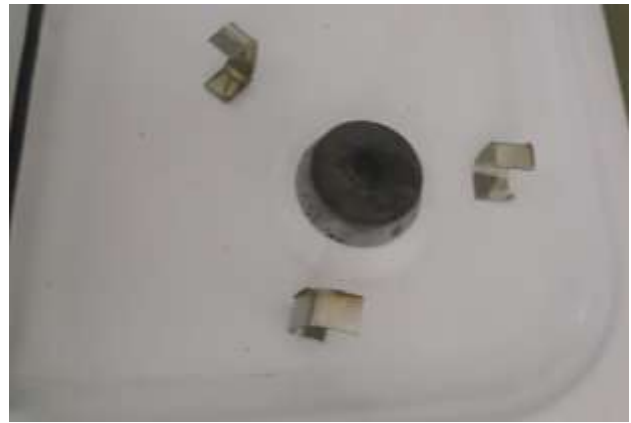
Figure 20. Image of newly developed attachments for a gas stove.
