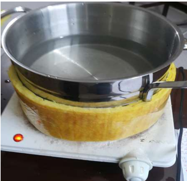
Figure 4. The image of a steel pot being insulated with sheet metal without using circular plates.
