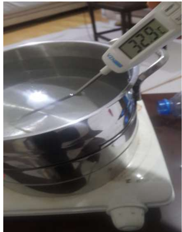
Figure 1. Photograph of an experiment showing temperature and time variations conducted by covering a steel pot with a circular sheet metal plate.
