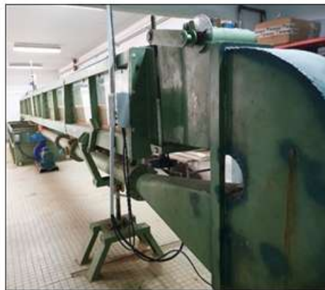
Figure 2: Photograph of the experimental set-up of a rectangular channel flume.
