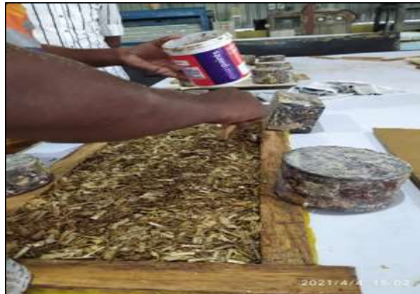
Figure 1 Fiber arrangement and compression molding process
