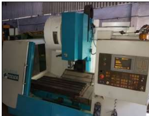
Figure 2: Vertical milling machine setup used for the drilling experiments
