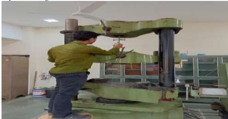
Figure 21: setting up a universal testing machine (UTM)
