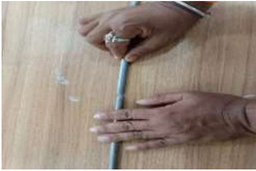
Figure 19: Torsion Test Specimen Inspection Before Testing
