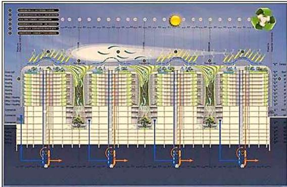
bottom - vertical section of the project, and the images show the increase in the percentage of the green component and the use of sustainable systems in the site, buildings and mass formations through the creation of shaded skylights with a negative design by attracting wind inside the buildings with shading of the facades by means of green facades and biometric facades, (Charkas 2019))
