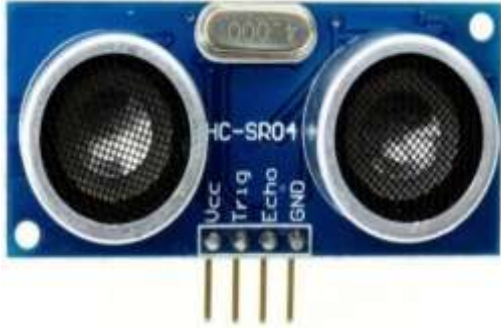
Figure 2. A popular low-cost ultrasound sensor: HC-SR04.
