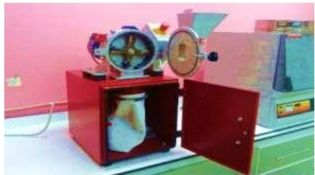
Figure 1. The humming machine for producing sawdust.
